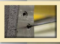
In-House Deep Hole Drilling Hole diameters as small as 3/16
